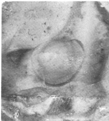
Figure 3. Autoradiograph showing uneven adsorption on an initially dry polyvinylpyridine surface. Rotated with bubble 48 hours at 37°C. Heparin concentration 638 \mu\text{g./ml.} , average heparin adsorption 7.6 \mu\text{g./cm.}^2 . Autoradiograph exposure 72 hours (comparable with Figure 2). In the lower third there is a fold or crack line in the film, probably introduced before the sack was made
